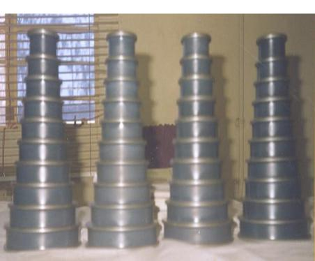
Stepper cone pulleys
